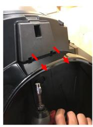
Remove meter backing. Turn the cap covering the USB port to the left to unlock and uncover the port. Insert the USB Maps card. Replace the cap and turn to the right to lock.
