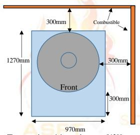
There must be a minimum clearance of 1200mm in front the door opening to combustible materials at all times.
