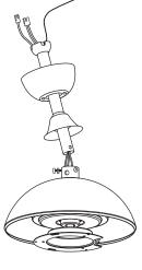
5. Insert the Down Rod into the Yoke making sure that the wires are not twisted and aligning the holes for the pin on the Down Rod with the holes in the motor Yoke. Insert Pin all the way through and put the Clip in place. Secure tightly the 2 Set Screws and Nut. Lower Yoke cover until it rests on the Motor Assembly.
