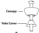
3. Loosen the Set Screw and Nut and the Set Screw on the Yoke.
