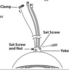
4. Thread the wires and Safety Cable that comes from the motor assembly through the Down Rod.
