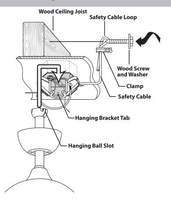
A WARNING: Failure to align hanging ball slot with hanging bracket tab may result in serious personal injury or death.
