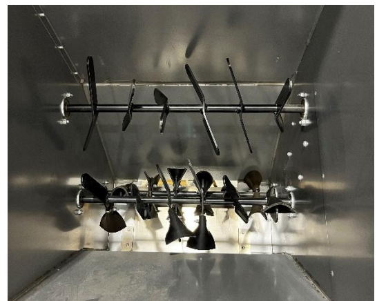
3 agitators provide for ideal product conditioning
