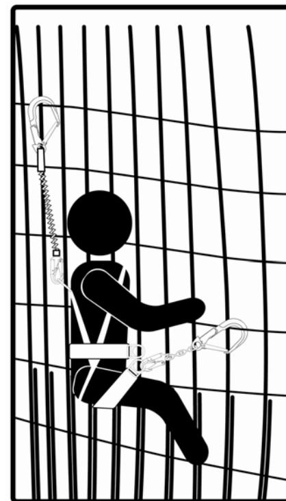
Correct Method for Work Positioning/Tower Work
