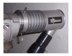
Make sure you utilize an industrial High Efficiency H.E.P.A. vacuum to contain any hazardous dust and debris. **Novatek** has a complete line of H.E.P.A. vacuums that will fit your needs.
