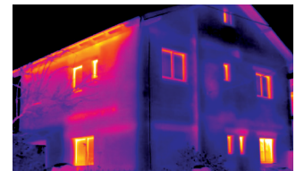
Detect energy losses from buildings: immediately identify and record thermal bridges in building fronts or shells.
