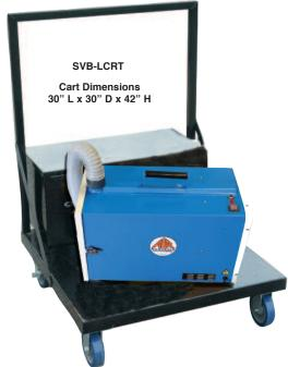
Optional Cart holds Model PFE-230 and provides a storage cabinet for welding supplies. Cart is made of steel with black powder coat paint, front swivel casters and rear locking casters.
