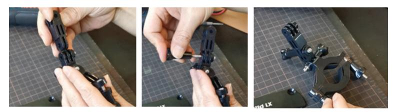
Put the two spacers into the two gaps of the extension piece's top respectively. Use a tool to adjust the hole and adjust accordinly so the circluar parts are aligned for the long screw to go through.
