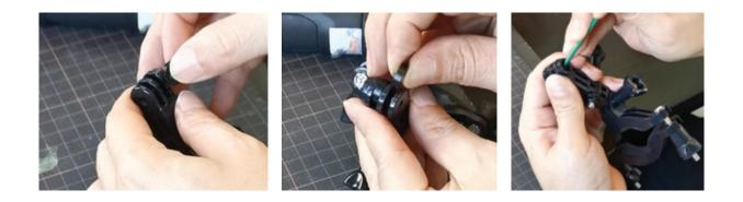
Insert the long screw to have it go through the right plate first and one-piece cyclinder, then carefully when inserting through the extension piece. Afterwards, complete the insertion through the left plate and tighten the screw.
