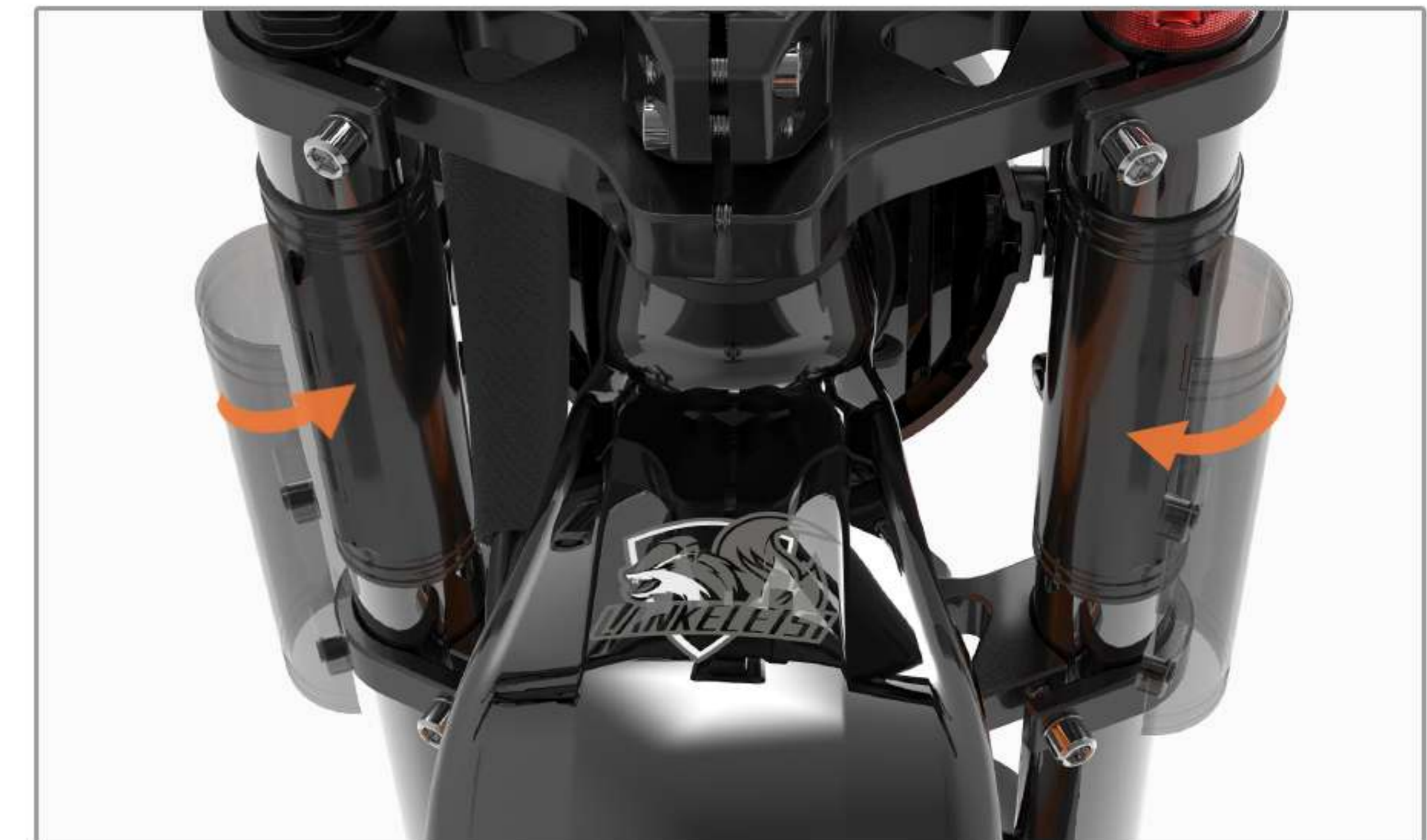
03 Attach the headlight to the fork
