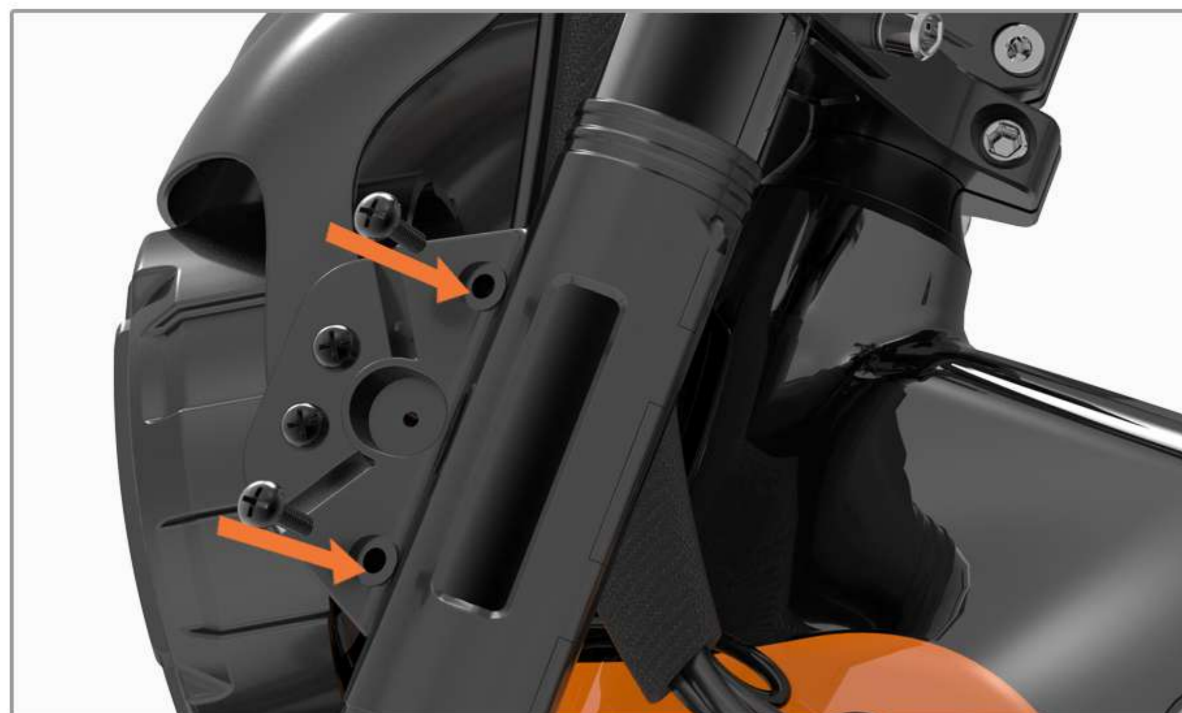
04 Insert the screws on both sides and lock them with the tool
