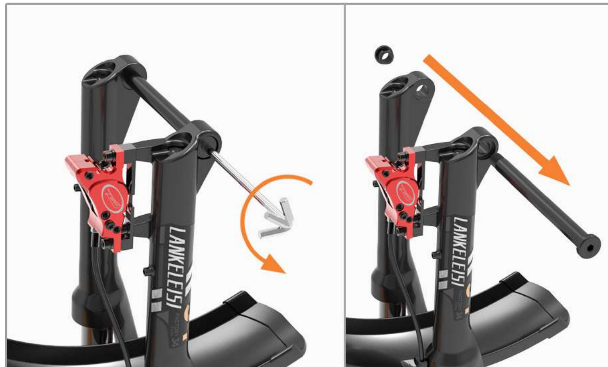
01 Remove front wheel mounting bearings
