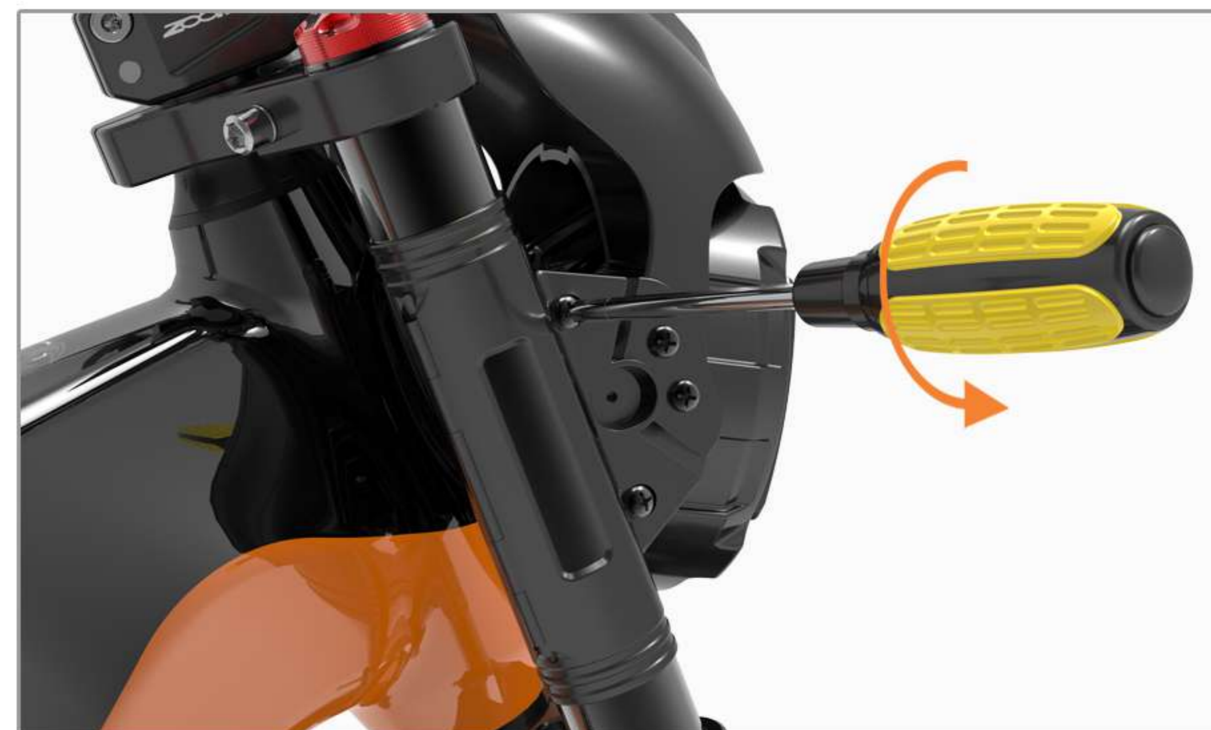
05 Locking screw, headlight installation completed
