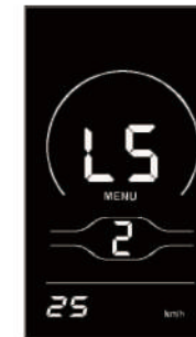
Fig. 7-2 Speed Limit Setting Interface
