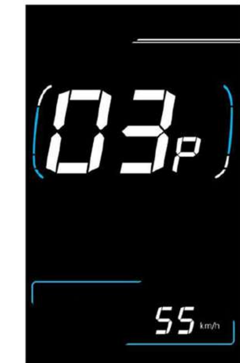
(03P is shown in the picture) Speed limit setting interface
