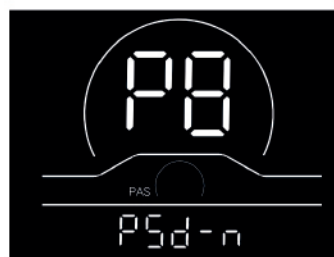
Fig. 4-8 Power-on Password Setting Interface
