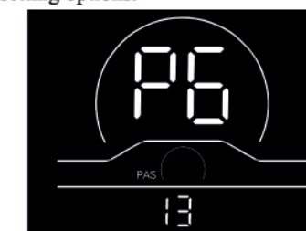
Fig. 4-6 Current Limit Setting Interface
