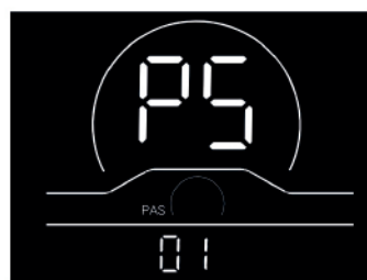
Fig. 4-5 Speed Sensor Setting Interface
