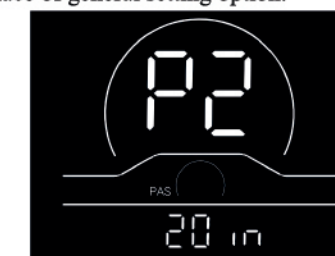
Fig. 4-2 Wheel Diameter Setting Interface
