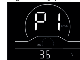
Fig. 4-1 Rated Voltage Setting Interface
