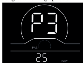
Fig. 4-3 Speed Limit Setting Interface
