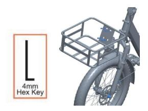
(2) Secure the shelf by clockwise installing the 4 bolts using a 4mm hex key.
