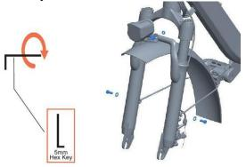
(2) Align the fender bracket with the headlight hole and the front fork fender pull hole. Insert the threaded end into the screw and tighten.
