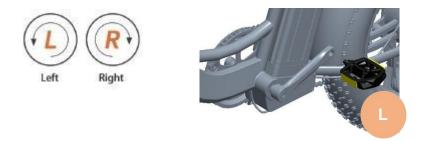
(2) Tighten the right pedal clockwise and the left pedal counterclockwise by using a 15mm wrench.
