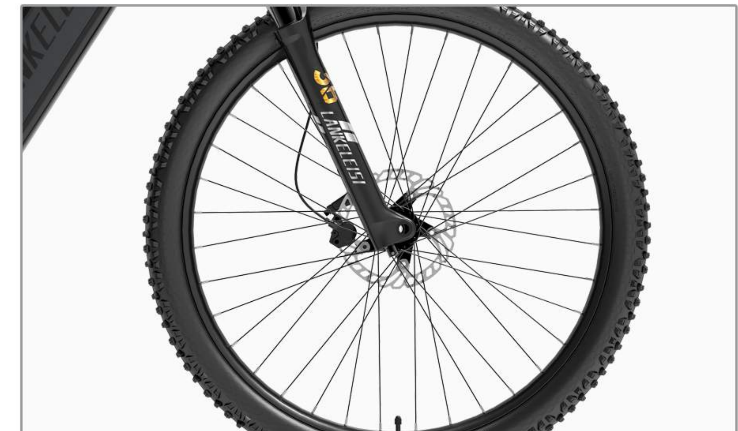
06 Install the front wheel centrally on the front fork
