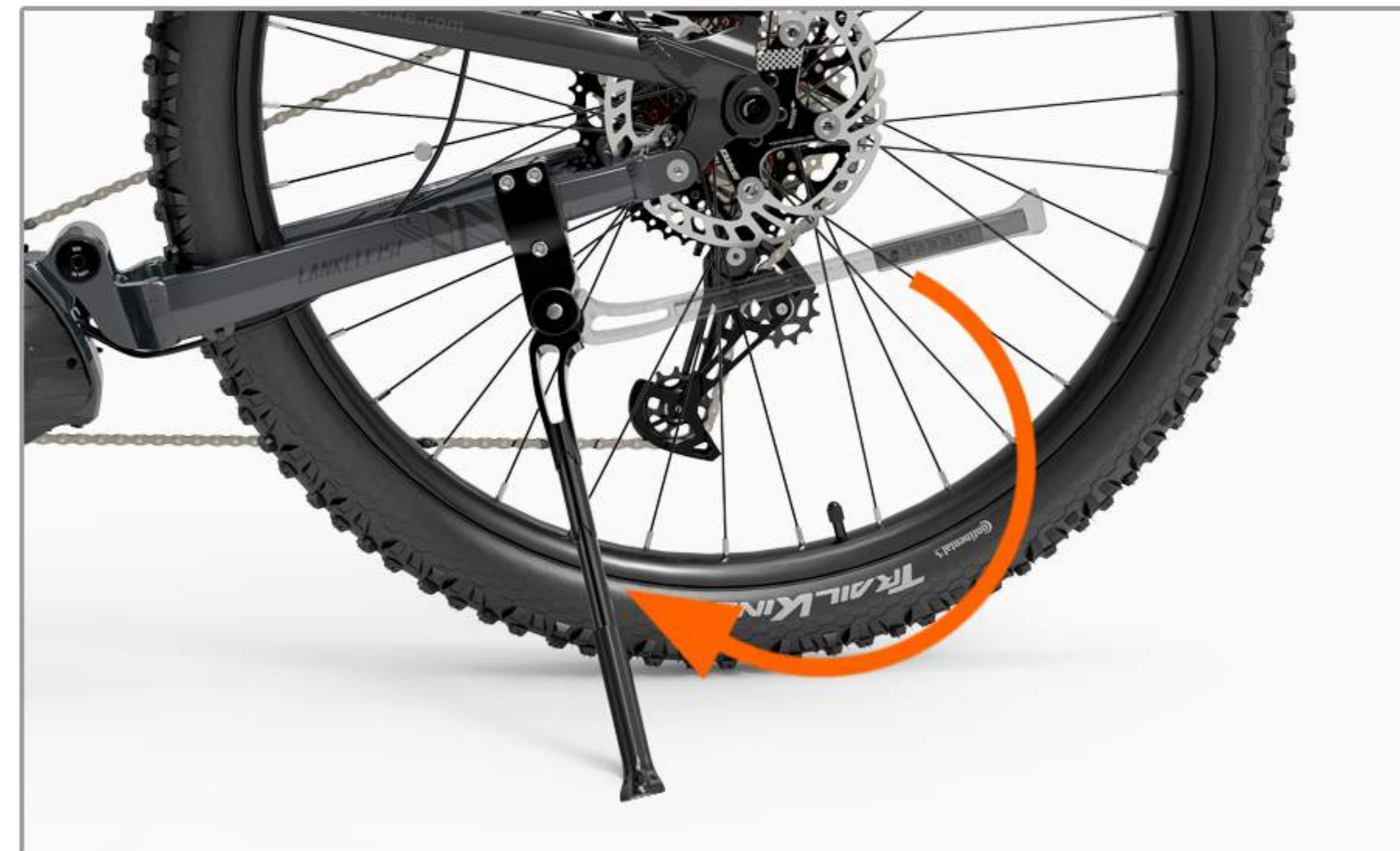
02 Lower the side supports and let them support the vehicle
