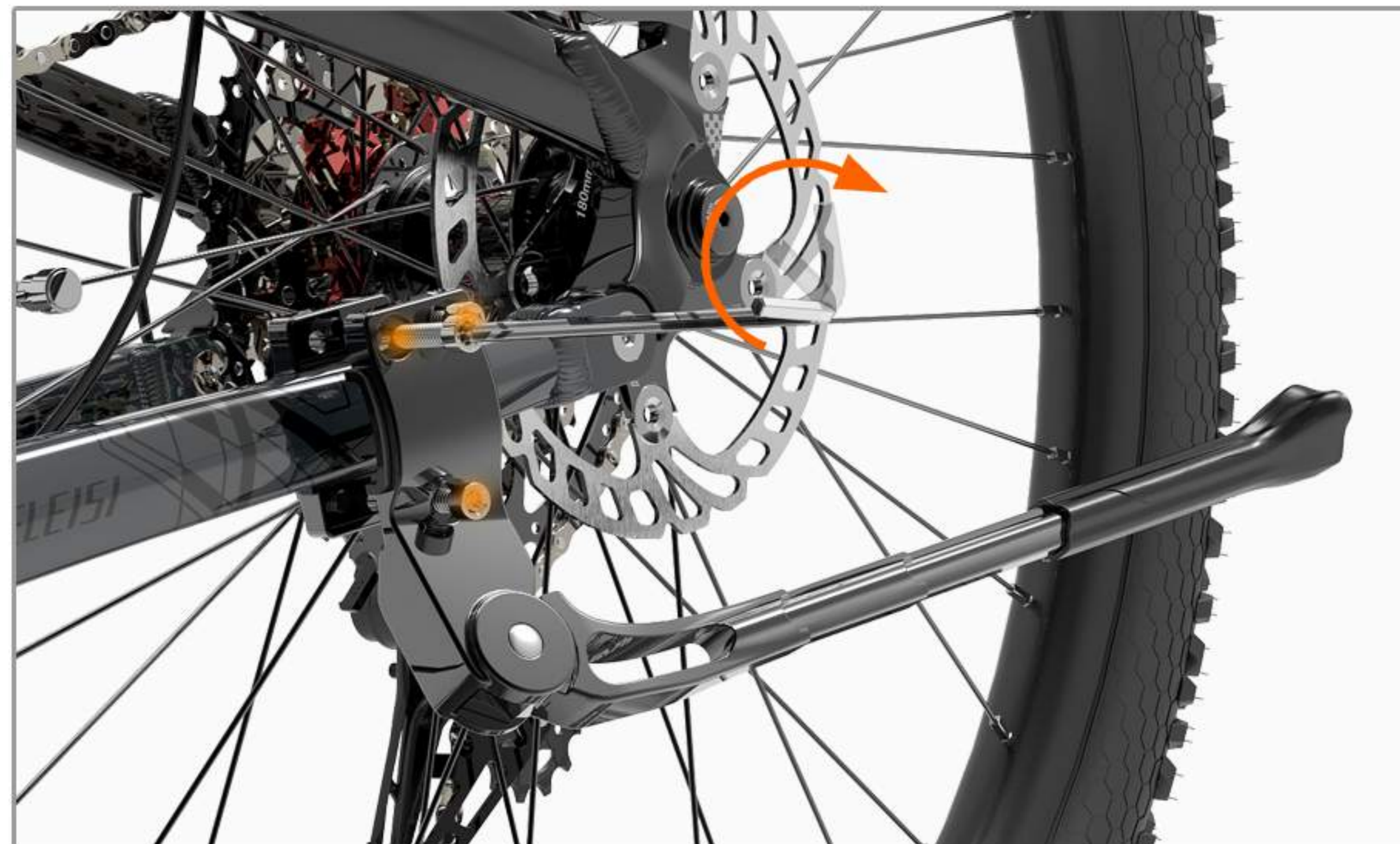
01 Hold the side supports in place and tighten the screws
