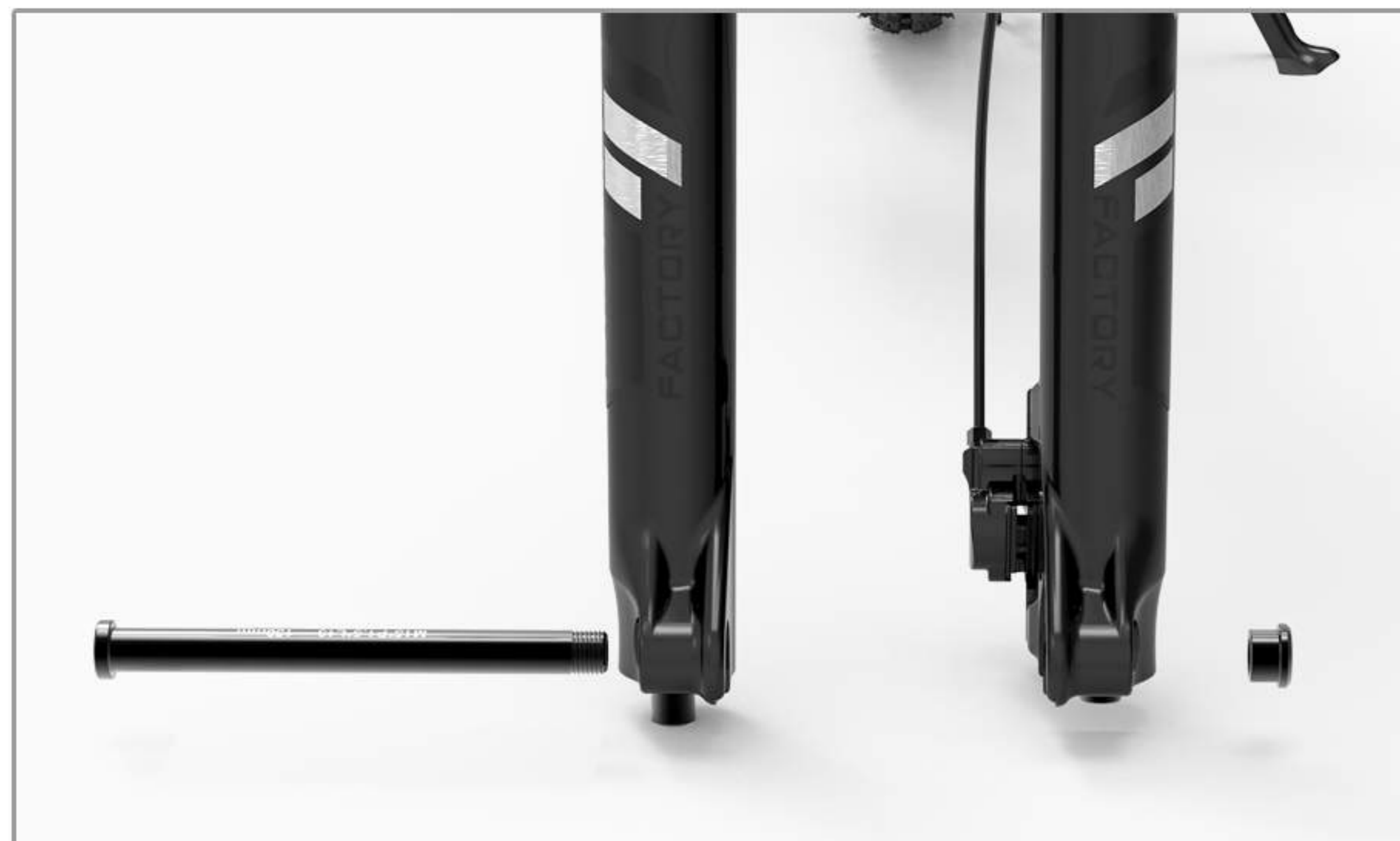
04 Remove the front wheel mounting shaft
