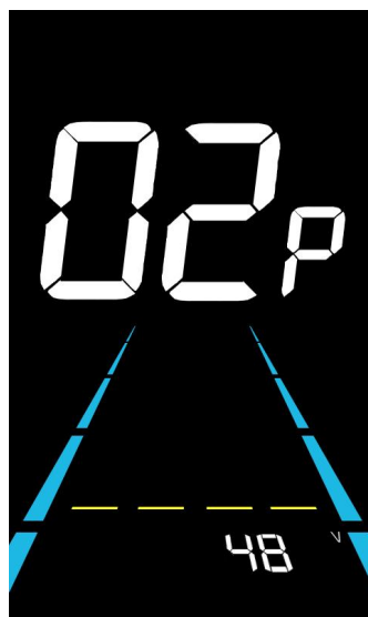
Figure 6-2 Rated voltage setting interface
