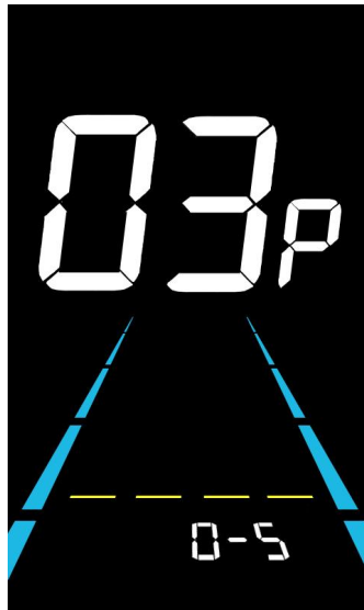
Figure 6-3 PAS level setting interface
