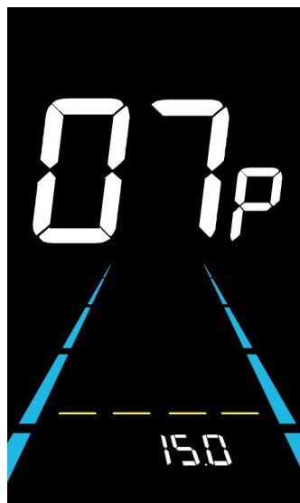
Figure 6-8 Controller current limit setting interface
