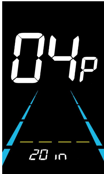
Figure 6-5 Wheel diameter setting interface
