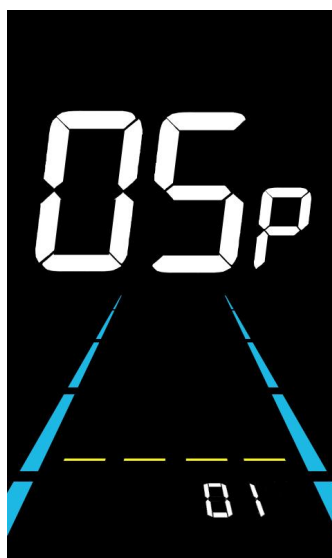
Figure 6-6 Number of speed sensor magnets setting interface
