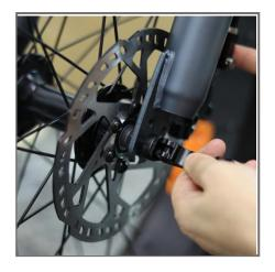
① Put the wheel in the front fork, insert the front fork axle, fix the screw
