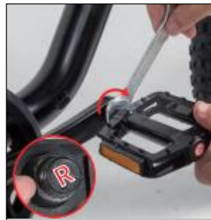
Step 02 Install the right foot pedal with a tool.
