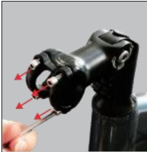
Step 01 Remove the four screws
