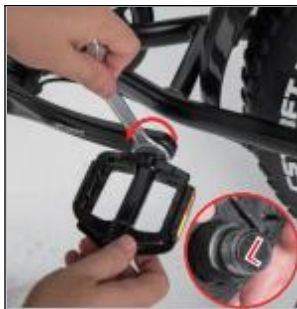
Step 01 Install the left foot pedal with a tool.
