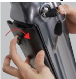
Step 02 With the other hand simultaneously lift the battery up.
