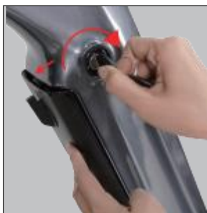
Step 01 Open battery lock with key.
