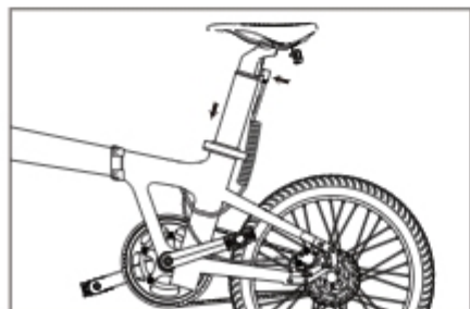
1.Insert the battery into the seat tube, then connect the battery cable
