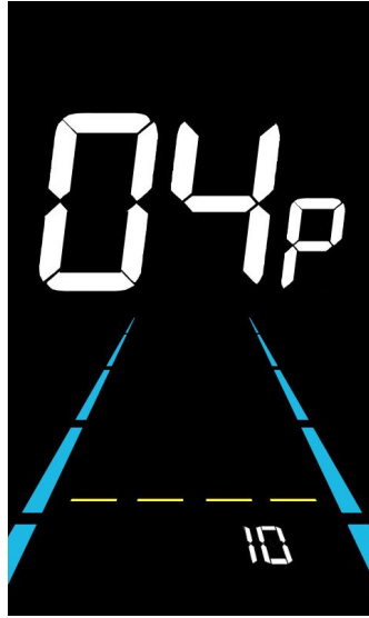
Figure 6-4 Auto Power Off Time Setting Interface
