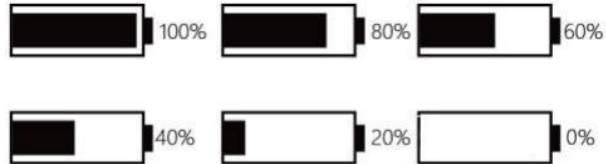
Battery SOC Indication Interface
