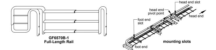
The Full Length rail, shown above, is a nominal, telescoping full length rail that provides maximum length rail perimeter coverage.
