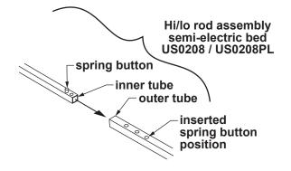
Depress spring button and insert inner tube into outer tube until third hole is reached as shown above. Release spring button to lock it into hole.
