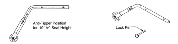
We recommend the use of anti-tippers at all times. The appropriate anti-tipper setting for your wheelchair's seat height is shown at above left.
