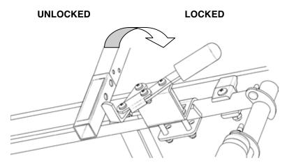
The Regency 5600 has two wheel locks — one on each rear wheel. To engage the wheel locks, push the levers forward until they lock into place, as shown above. To disengage, pull back on the levers until the wheels roll freely.
