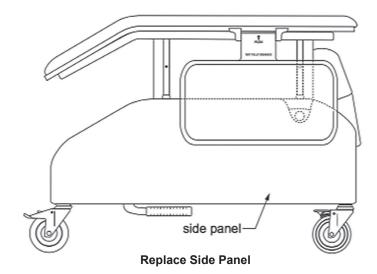
10. Re-install side panel: insert side panel into recliner frame by lining up side panel clips with frame tubes. Push side panel firmly into frame until side panel clips lock into place.
