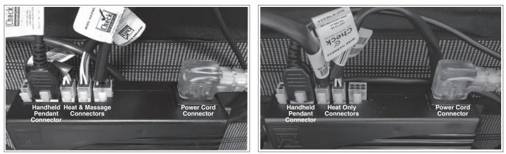
Heat and Massage Feature – Control Module and Transformer Unit Showing All Connections Correctly Made Heat Only Feature – Control Module and Transformer Unit Showing All Connections Correctly Made
