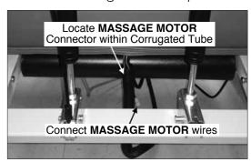
**Connect Massage Motor Wires**
