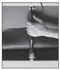
**Adjusting Cable Tension 1**
