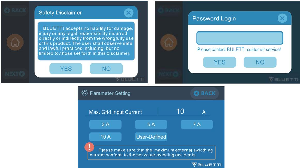
**Note:** The Grid Input Current is set at 10A by default. The change only takes effect when AC300 connects to the grid.
