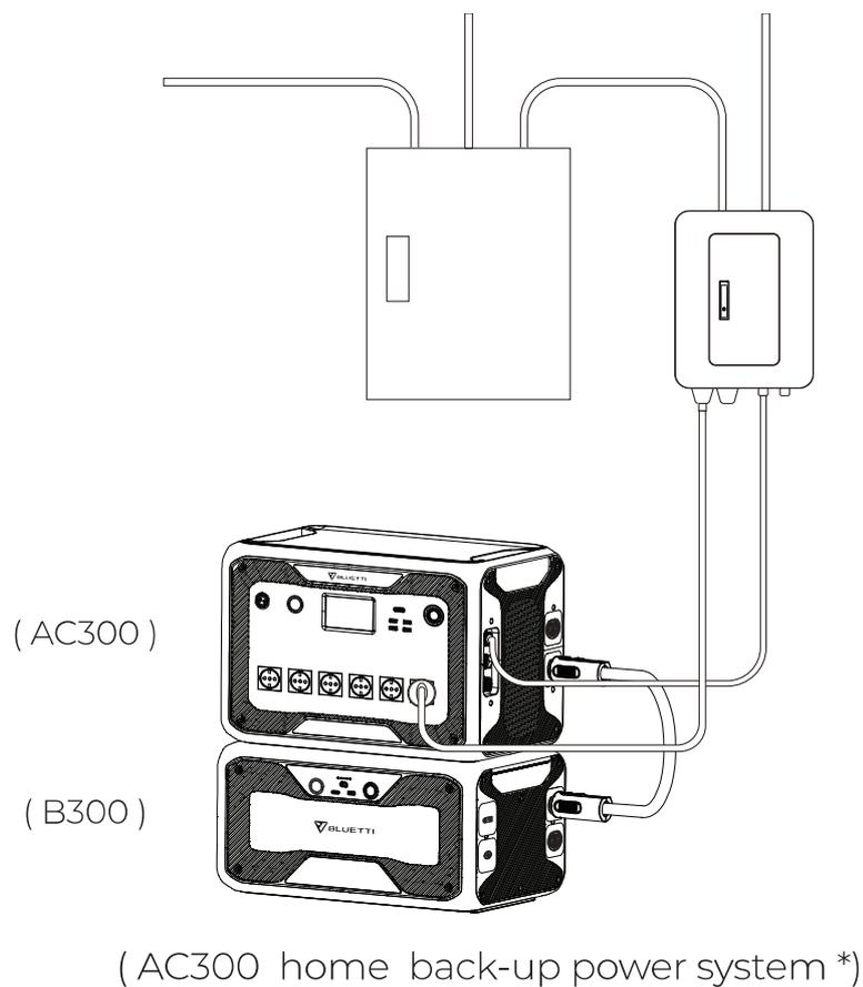
\* **Note:** For more details, refer to “How to build a partial-home backup system with AC300+B300” .
