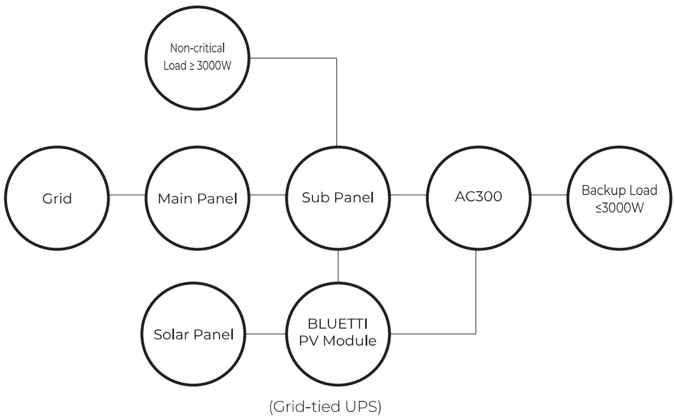
**Note:** Refer to “How to build a partial-home backup system with AC300+B300” for more details about Grid-tied UPS.
