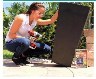
**Step 1:** Drill a hole on the bottom of the planter using the 1-1/4 in drill bit.
