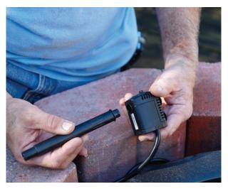
**Step 3:** Add Complete Filter Kit with Pump. Fill the rigid liner with water to 2 in. below the top of the liner.
