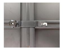
Step 7: Slide the M8 bolt and plate set into the mounting track, then secure it by inserting the M8 bolt through the U bracket. Repeat for each corner of the tent.
