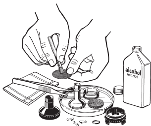
Manual cleaning with isopropyl alcohol (70 %) or detergent
