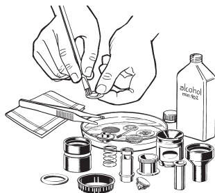
Manual cleaning with isopropyl alcohol (70 %) or detergent
