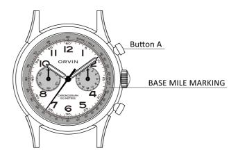
This function enables users to determine average speed based on a measurement of the amount of time it takes to travel a certain distance (1 mile). It can also be used to determine the rate of production per unit of time (per hour). (measuring range: maximum 60 seconds)
