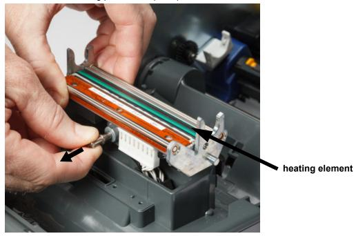
4. Rotate the printhead to expose the cables. Note the orientation of the cables so that you attach them to the new printhead in the same orientation.
