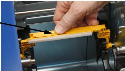
3. Slide the wiper pad to the left until it pops out of the wiper arm.
