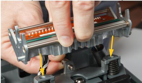
7. While pulling the pin out, set the new printhead on its mounting.
