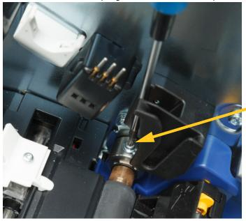
9. Reinstall the two screws on the yellow disk in the access hatch. Take care not to overtighten the screws.
