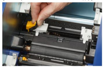
8. Pull the leading edge of the labels from the top of the roll until it sits just past the black rubber roller, but no further. For wide labels, be sure to feed them under the label supply guides.
