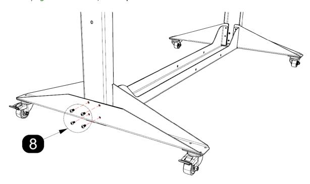
c) Screw 4x M6 Bolts 3 through the Foot 2 into the holes on the inside of the Frame Upright 1 at one end, then repeat this at the other end of the Bottom Rail 3.
