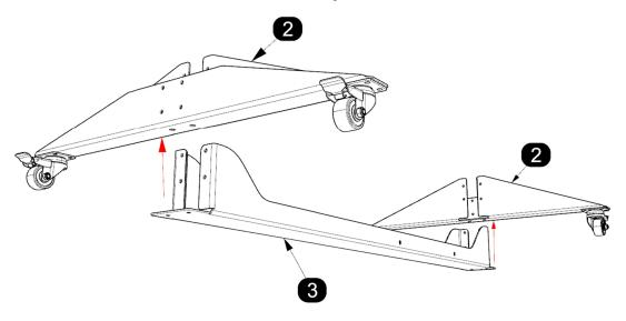
b) Screw 2x M6 Bolts 3 into the underside of the Foot 2 using the 5mm Allen Wrench. Repeat this for the second Foot 2 at the other end of the Bottom Rail 3.Be careful not to over-tighten the bolts.
