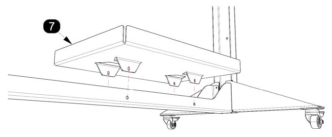
b) Screw 4x M6 Bolts 3 through the tabs of the Reservoir Tray 6 (2x M6 Bolts 3 each side) into the Bottom Rail 3.
