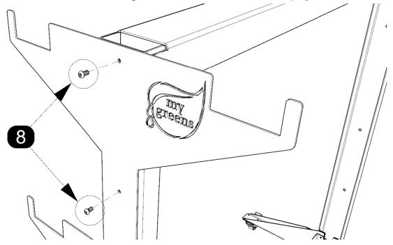
d) Place End Plate B **6** against the Frame Upright **1** closest to the reservoir tray and align the bolt holes.
