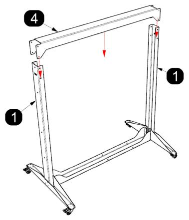
b) Screw 2x M6 Bolts 3 through one end of the Top Rail 3 into each side of the Frame Upright 1. Repeat this at the other end of the Top Rail 4.
