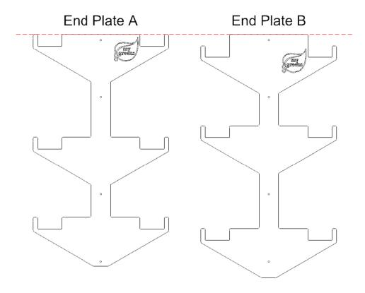
b) Place End Plate A **9** against the Frame Upright **0** closest to the reservoir tray and align the bolt holes.
