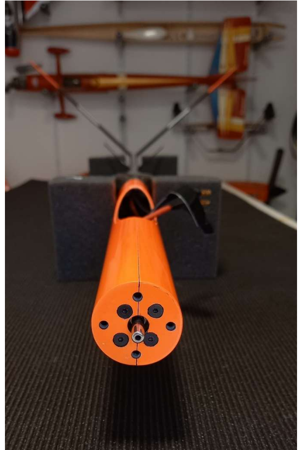
Replacement of the screw holding the fuselage servo plate (black Hex key)
