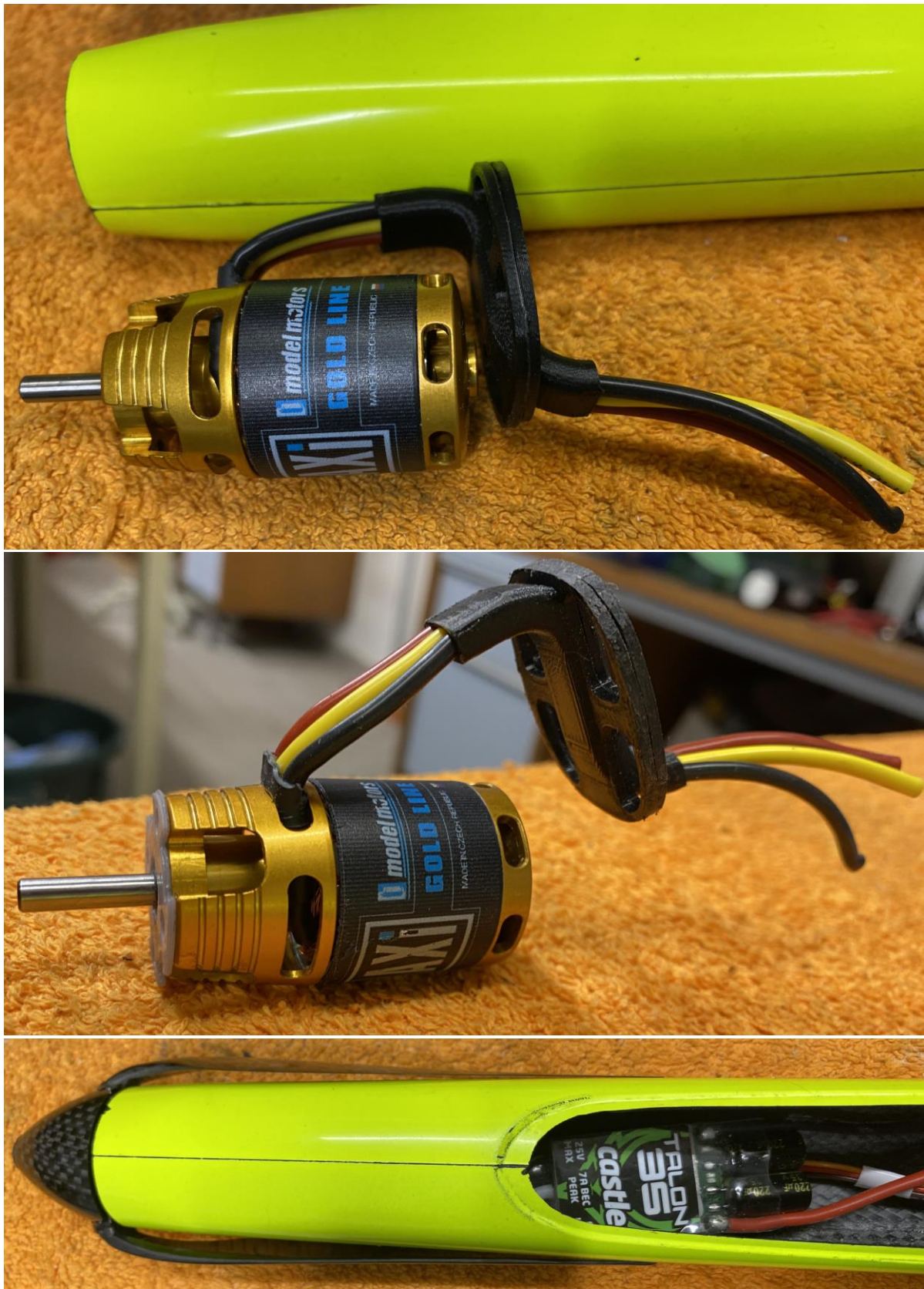
Figure 13: ready assembled motor unit before placed into nose cone
