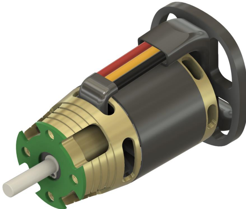
Figure 11: mounted motor unit ready to place into nose cone
