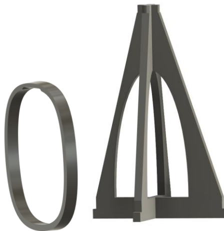
Figure 5: Spar position ring with helper tool for positioning
