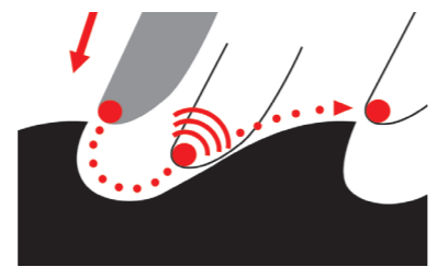
Automatic probing of the grinding wheel at the saw tooth
