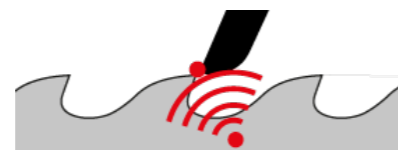
Automatic tracing at the tooth with vibration sensor (impact sound sensor)
