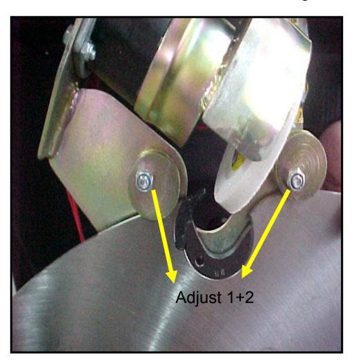
Adjust grinding wheel to correct height and face angle by loosening Nut 1 & 2 and adjusting rolls to correct position.
