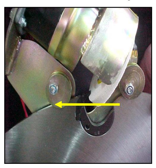
➤ When required adjustment is set, roll grinding wheel onto face of tooth. This setting will be same for all teeth on saw.
