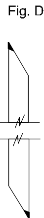
Figure D illustrates the knife depth of a balanced head with equal amounts of knife tip being removed in the jointing process.
