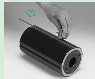
Put the setting jig between block and back plate to make a space so that the knife will be easily slide in.
