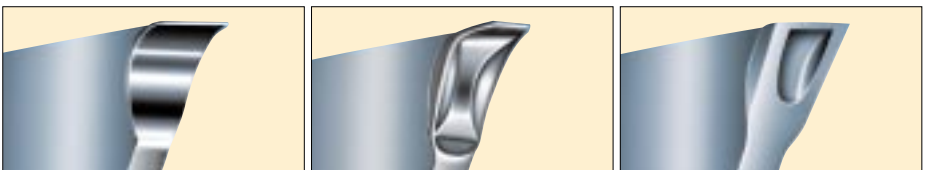
Upset tooth point, side-dressed tooth point and finished tooth point.
