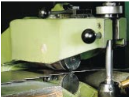
Rolling of bandsaw blade.
