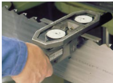
Checking the tooth symmetry.
