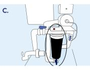
Locate the particle filter housing. It will have a black sock over a plastic chamber.
