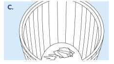
Use a wet vac, or clean mop/cloth, to catch and remove any debris from the bottom of the barrel. This is also a good time to replace the particle filter.
