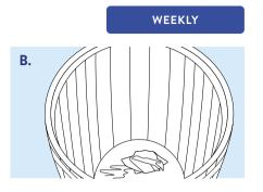
Using a clean cloth (or wet vac), reach into the water and catch any debris caught on the mesh gauze sat over the suction hole.
