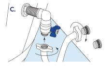
Take the other hose. Attach one end to the return flow hole tap and the other to the connector marked 'Outlet'.
