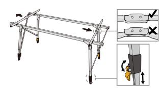
Filp the table up and adjust the height using the yellow level.
