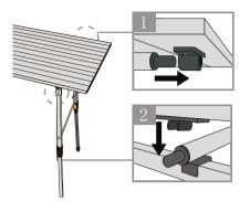
Slide in the tabletop at one end and press down the other end to click into place.
