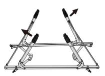
Place the frame facedown on the floor, Pull the four legs outwards and facing up until fully extended.
