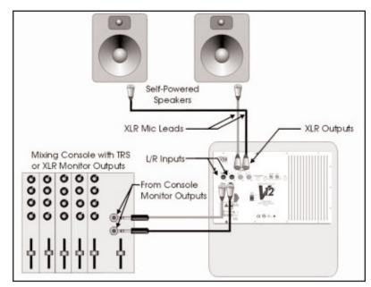
If you are using active (powered) speakers, simply use an XLR male to female "mic lead" to connect the output of the subwoofer directly to the input of the speaker. The output marked "Left" should go to your left speaker, and the output marked "Right" should go to your right speaker
