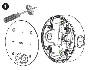
Remove the plastic cover and seal ring from the conduit hole you want to use, and install them the conduit hole you don't want to use to make sure the bracket is waterproof.
