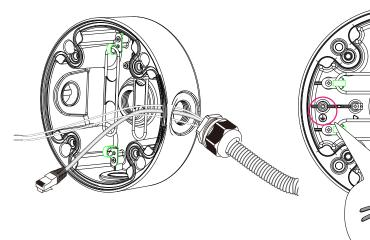
Secure the camera top cover. Connect a ground wire to this position.
