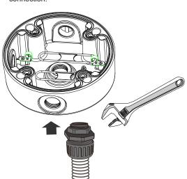
Install the cable gland and pass cables through it.
