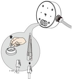
Connect cables to the Ethernet port and terminal block.
