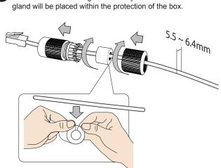
Install the waterproof components of the cable gland to your Ethernet cable following the QIG of your camera. The cable
