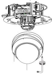
7. Use a #2 Phillips screwdriver to loosen the clamping plates (see drawing below) and insert the recessed-mount bracket through the hole in the ceiling.
