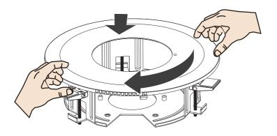
5. Install camera to the recessed-mount bracket by driving screws.
