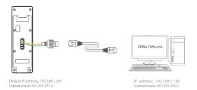
Click on [COMM.] > [Ethernet] > [IP Address], input the IP address and click on [OK].
