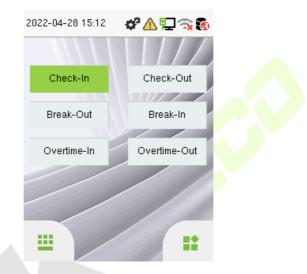
Press the corresponding punch state key to select your current punch state, which is displayed in green. Please refer to "Shortcut Key Mappings" for the specific operation method.
