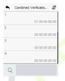
On the combined verification interface, tap the Door-unlock combination to be set, and tap the **up** and **down** arrows to input the combination number, and then press **OK**.
