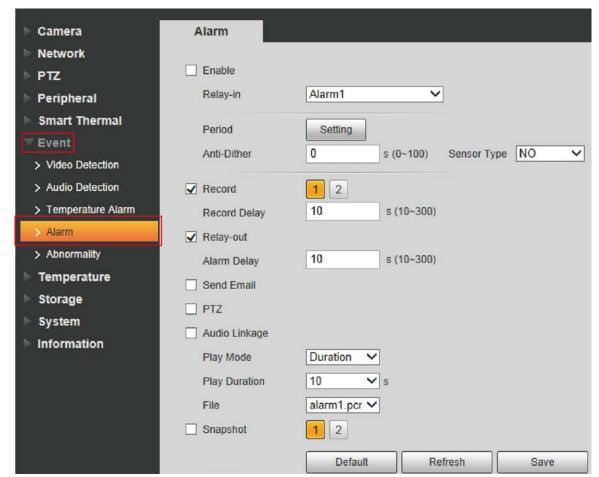
Figure 5-1 The alarm interface
