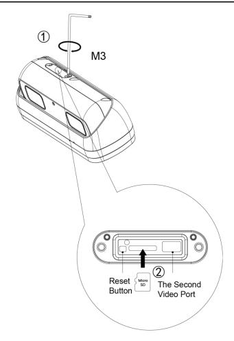
Press the reset button for 10 seconds to reset the device.
