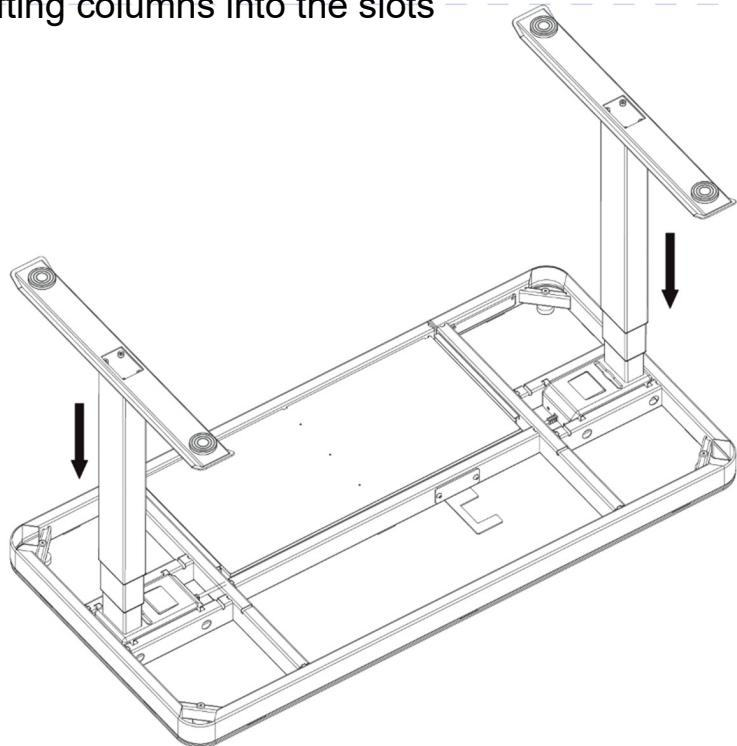
2.2 Tighten the 8 Pre-installed Screws (E) to attach the lifting columns to the table top
